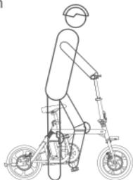
Fold the kickstand, open the power switch and step on the pedal one foot by one foot.
